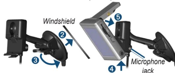
To remove the nüvi from the cradle, press the small tab on the bottom of the cradle up, and tilt the top of the nüvi forward.
