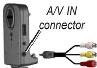
2. Connect the red, white, and yellow connectors to the corresponding plugs on your video device.
