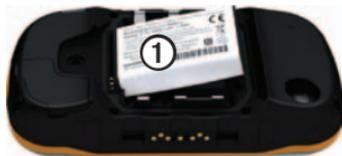
3. Align the metal contacts on the battery with the metal contacts in the battery compartment.
