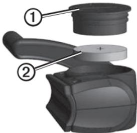
2. Use a coin to twist the cover counter-clockwise until it is loose enough to remove (arrow points to unlocked).
