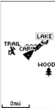
When you select 'Orient Map Northwards' the figure icon is replaced by a 'direction' triangle. The tip of the triangle tells you the general direction you are moving.
