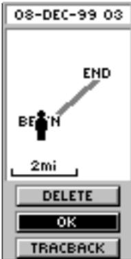
The 'BEGIN' point is the point defining the starting point when saving a track log. 'END' is the last point that was saved. Each saved track will always have a 'BEGIN' and 'END' point for navigation. The 'BEGIN-END' pair imply the direction of the saved track. If you want to retrace the track, navigate to 'END'. If you want to track back to the starting point, navigate to 'BEGIN'.
