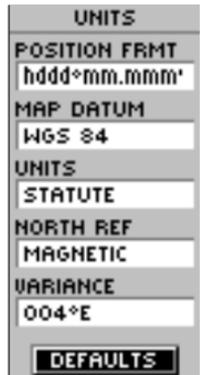
The 'DEFAULTS' setting will reset the eTrex units to all of its factory settings.
