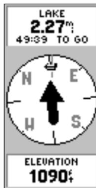
*The Pointer Page allows you to display eleven types of different data, such as ‘Elevation’.*
